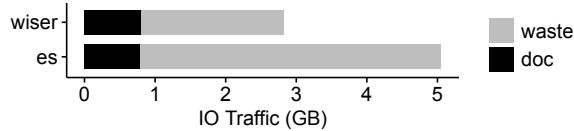
Figure 12: Document Store Traffic doc indicates ideal traffic size. The relative quantity between Elasticsearch and WiSER is the same across different workloads; therefore, we show the result of one workload here for brevity (single-term queries with the popularity level = 10).
