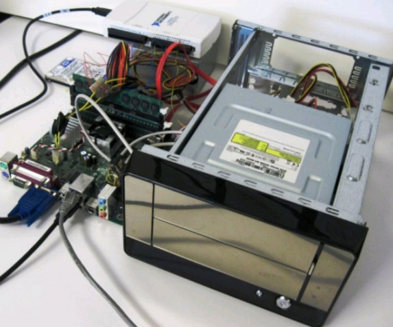
Figure 1: Atom LEAP next to case, with DAQ behind.
