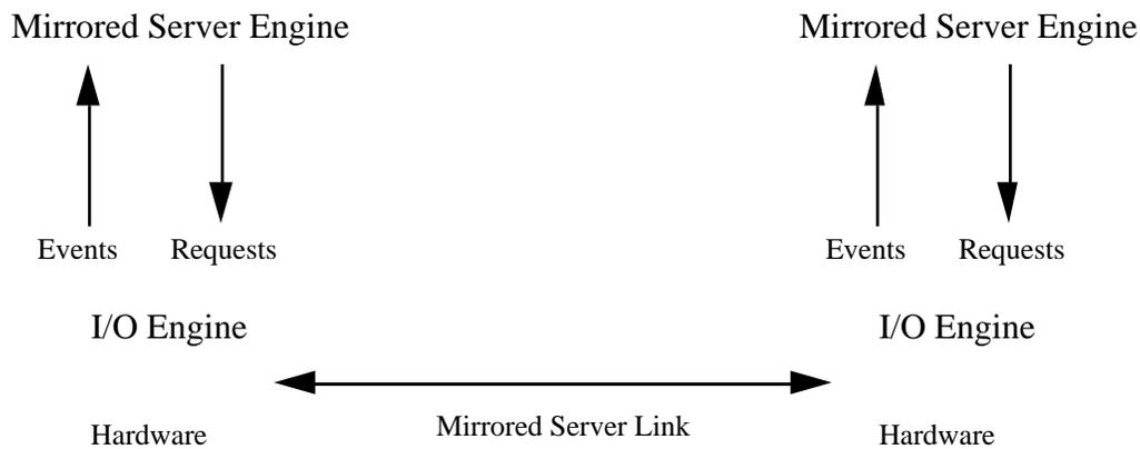
At the moment of starting, the state in both mirrored server engines is identical. Server mirroring works by keeping the state of the two mirrored server engines identical over time, so that if the primary dies (because of a hardware failure, say), the secondary engine will be able to take over (with almost no action required on the part of the clients<sup>10</sup>).
