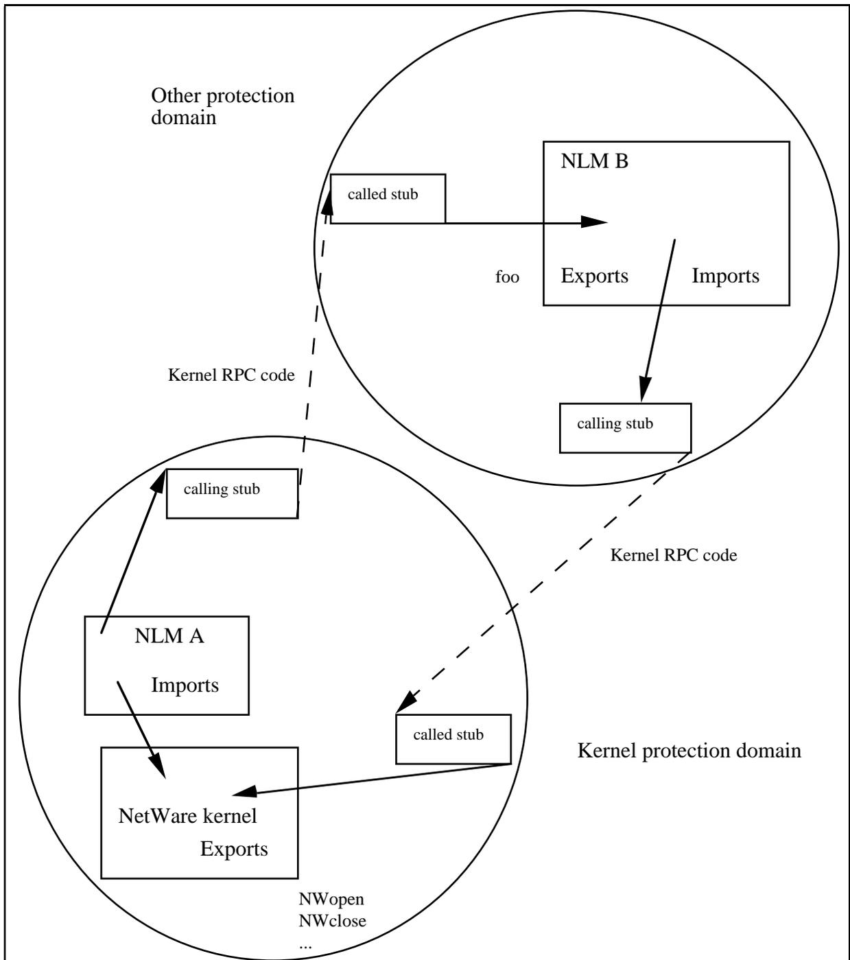
In this figure, NLM A is importing one routine from the kernel and another ("foo") from NLM B. NLM B is also importing one routine from the kernel.
