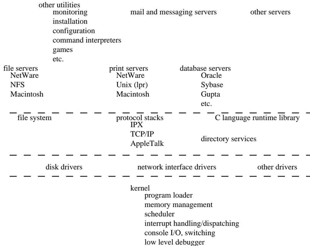
Outside of the kernel, each separate piece in the above figure consists of one or more NLMs. Thus, NLMs can be device drivers, higher level parts of the operating system, server processes, or utilities.
