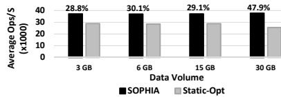
Figure 8: Effect on increasing data volume per node. We use a cluster of 4 servers and compare the performance to the static optimized. The results show that SOPHIA’s gain is consistent with increasing data volumes per node.
