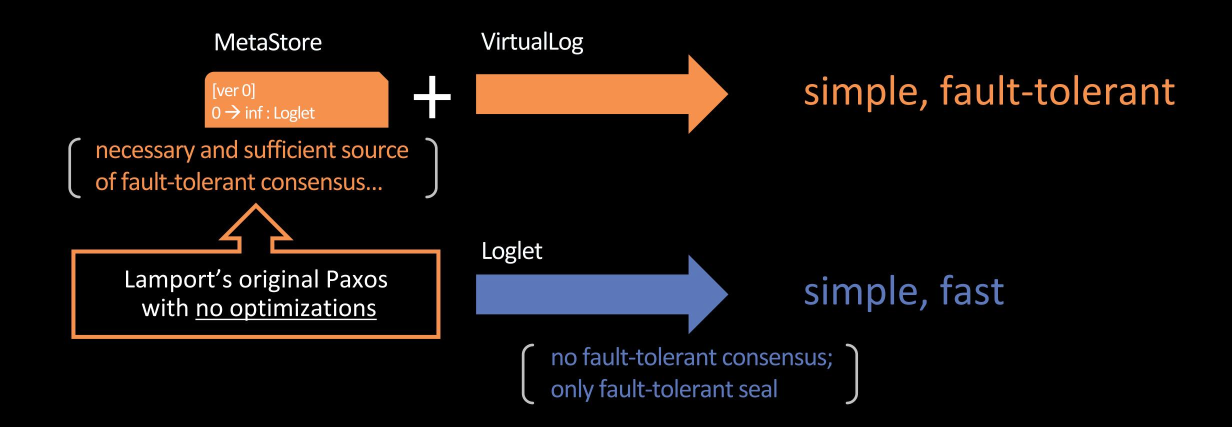
the VirtualLog handles all reconfiguration (including leader election); the Loglet provides failure-free ordering
