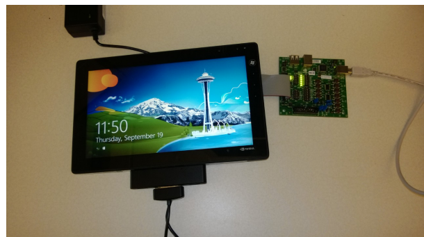
Figure 3: Windows RT 8.1 power profiling setup #2: Pre-instrumented to gather fine-grained power numbers for a smaller set of power rails including the CPU, GPU, Screen, WiFi, eMMC, and DRAM.
