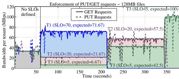
(a) 1 proxy/3 storage nodes, bandwidth control at proxy.
