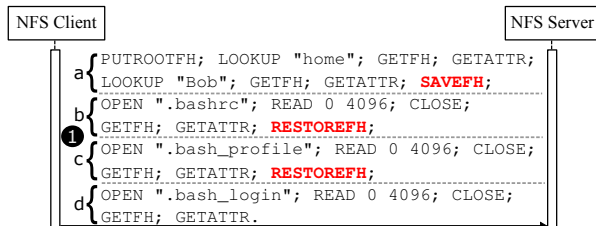
Figure 3: One NFS compound that reads three files. The operations can be divided into four groups: (a) sets the current and saved filehandle to /home/Bob ; (b), (c), and (d) read the files .bashrc , .bash_profile , and .bash_login , respectively. SAVEFH and RESTOREFH (in red) ensure that the CFH is /home/Bob when opening files. The reply is omitted.
