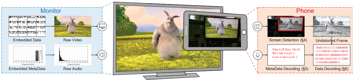
Figure 1: System overview of AIRCODE. The monitor displays a video with embedded data in raw video frames, and metadata (control information) in raw audio signals. The phone records the video, then detects screen in camera images to equalize distorted video frames, decodes metadata from audio signals, and finally decodes data embedded in video.
