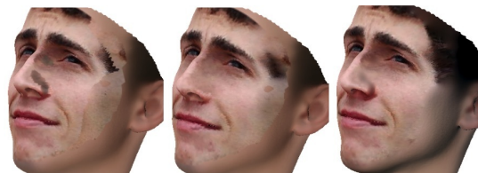
Figure 5: Naïve symmetrical patching (left); Planar Poisson editing (middle); 3D Poisson editing (right).
