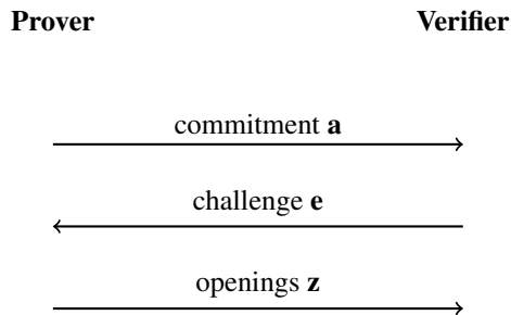
Figure 1: The communication pattern of a \Sigma -protocol.
