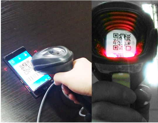
Figure 15: The masked QR code is being scanned and the reflection image of the masked QR code is captured by the malicious app with front camera.
