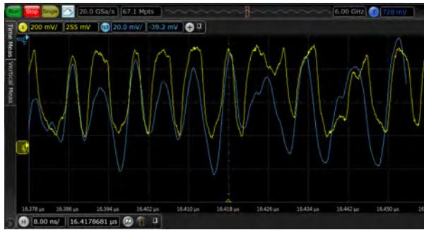
Figure 10: USB 2.0 data line crosstalk leakage from a hub of the same make as the one used in Figure 6. The yellow (top) trace shows the USB traffic and the blue (bottom) trace shows the observed data line crosstalk leakage measured from an adjacent downstream port (manually aligned with the yellow trace by subtracting 4ns).
