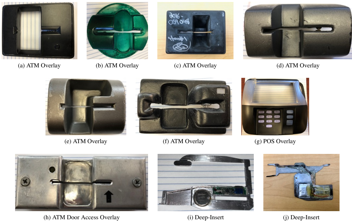
Figure 13: This figure shows the 10 real skimmers provided to us from the NYPD. The Skim Reaper successfully detected all of these skimmers.
