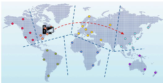
Figure 4: Illustration of Redirection Hijacking with Regional Anycast. (The global platform is divided into different regions, each of which leverages the anycast routing within the region. A redirection hijacking can force end-users to access the suboptimal or unresponsive edge servers located within a remote region.)
