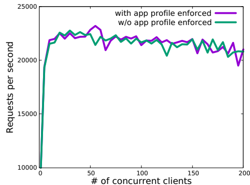
Figure 9: Throughput of containerized Apache with and w/o application AppArmor profile enforced.
