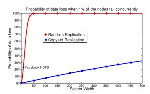
Figure 3: Data loss probability when 1% of the nodes fail simultaneously as a function of S, using N =5000, R = 3.
