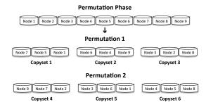
Figure 4: Illustration of the Copyset Replication Permutation phase.
