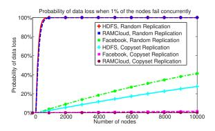
Figure 6: Data loss probability of random replication and Copyset Replication with R=3, using the parameters from Table 1. HDFS has higher data loss probabilities because it uses a larger scatter width (S=200).
