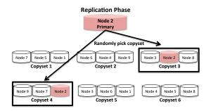
Figure 5: Illustration of the Copyset Replication Replication phase.
