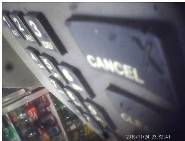
Figure 4: This is a frame of video captured by a camera deployed alongside a skimmer. The adversary uses the camera to capture the victim’s PIN upon entry. With both card data and the PIN, the card can be used to obtain cash.
