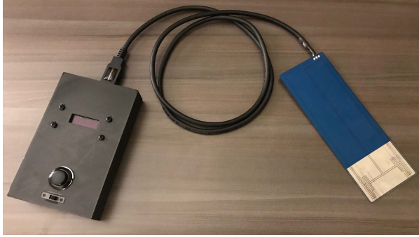
Figure 9: This is the entire Skim Reaper device, consisting of the microcontroller system (left) and the measurement card (right). The card is inserted into a card acceptor, where the number of read heads is measured by the microcontroller. After the user indicates that the test is complete, the user is notified if a skimmer was detected.
