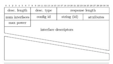
**Figure 3:** Bit-level description of message sent during bus enumeration from device to host containing configuration descriptors
