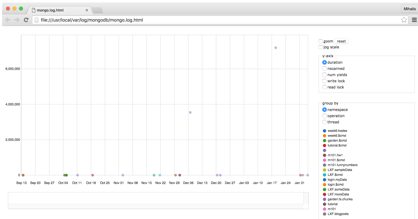
Figure 2: The output of the mlogvis Python script on a log file from my local MongoDB server
