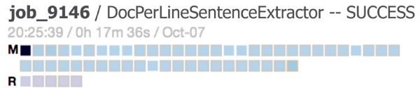
Figure 4: Visual signature of data skew. A node with anomalous task durations (darker color) and high volume of I/O (nodes are sorted by decreasing order of I/O) can signal data skew.
