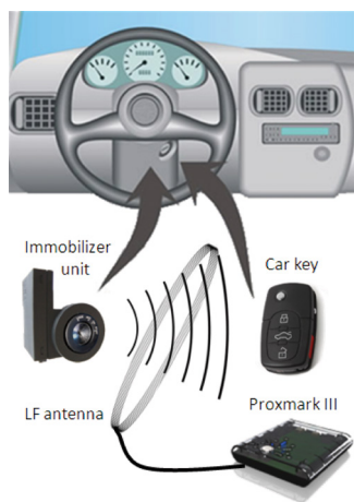
Figure 2: Experimental setup for eavesdropping
