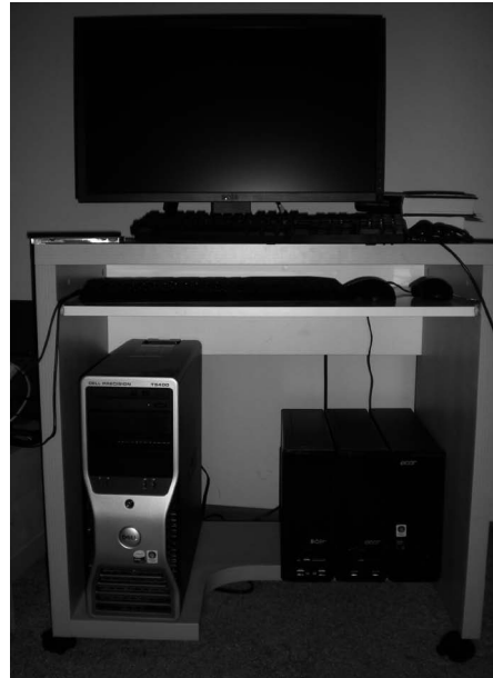
FIGURE 2. HYDRA, A MINIATURE CLUSTER WITH ONE MASTER PC AND THREE NODES, IS THE FIRST AUTHOR'S PRIVATE CLUSTER FOR HOME OFFICE USE. THIS IS ONE OF A SERIES OF INSTALLATIONS OF VARYING SIZES WE HAVE BEEN WORKING ON.
