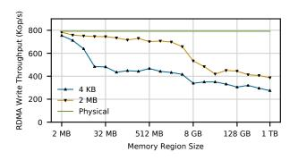
Figure 2: **RDMA Write performance over different memory region sizes.** This figure shows the throughput of 8-byte RDMA writes affected by the pin-down cache misses. Data measured on Intel Optane DC Persistent Memory with an Mellanox CX-3 RNIC.
