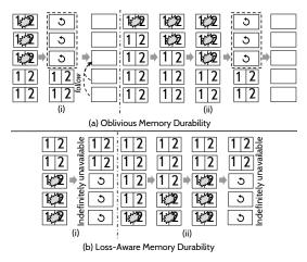
Figure 1: **Problems in Memory-Durable Approaches.** (a) and (b) show how a data loss or an unavailability can occur with oblivious and loss-aware memory durability, respectively. In (i), the nodes fail simultaneously; in (ii), they fail non-simultaneously, one after the other.
