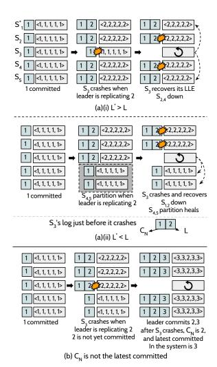
Figure 4: LLE Recovery. The figure shows how L' may not be equal to L. For each node, we show its log and LLE-MAP. The leader  $(S_1)$  is marked \*; crashed nodes are annotated with a crash symbol; nodes partitioned are shown in a dotted box; epochs are not shown.
