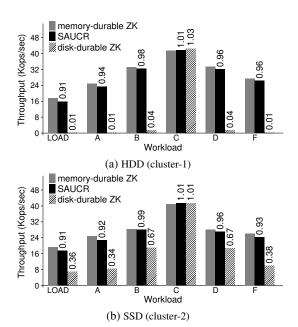
Figure 8: Macro-benchmarks. The figures show the throughput under various YCSB workloads for memory-durable ZK, SAUCR, and disk-durable ZK for eight clients. The number on top of each bar shows the performance normalized to that of memory-durable ZK.
