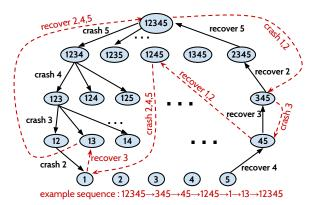
Figure 6: Cluster-State Sequences. The figure shows the possible cluster states for a five-node cluster and how cluster-state sequences are generated. One example cluster-state sequence is traced.
