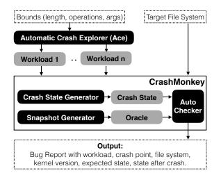
Figure 2: **System architecture**. Given bounds for exploration, ACE generates a set of workloads. Each workload is then fed to CRASHMONKEY, which generates a set of crash states and corresponding oracles. The AutoChecker compares persisted files in each oracle/crash state pair; a mismatch indicates a bug.
