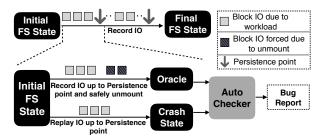
Figure 3: **CRASHMONKEY operation**. CRASHMONKEY first records the block IO requests that the workload translates to, capturing reference images called oracles after each persistence point. CRASHMONKEY then generates crash states by replaying the recorded IO and tests for consistency against the corresponding oracle.
