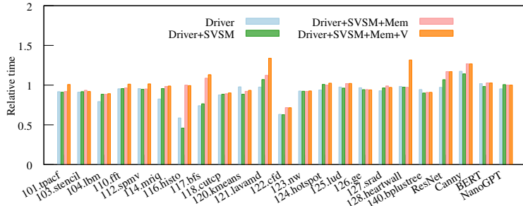
Figure 5: Relative execution time for the five benchmark suites evaluated on Honeycomb.
