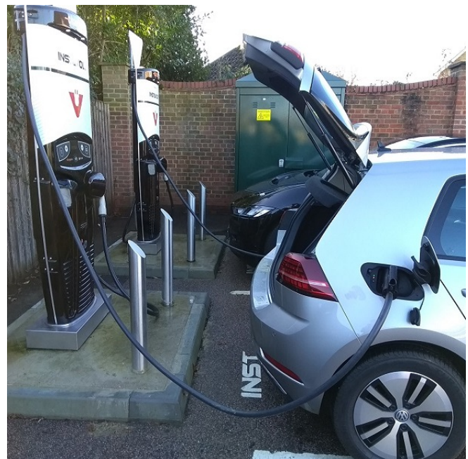
Figure 8: Two vehicles charging simultaneously. With the eavesdropper between the two vehicles 42.5% of messages were received successfully, including the NMK key establishment for both vehicles.
