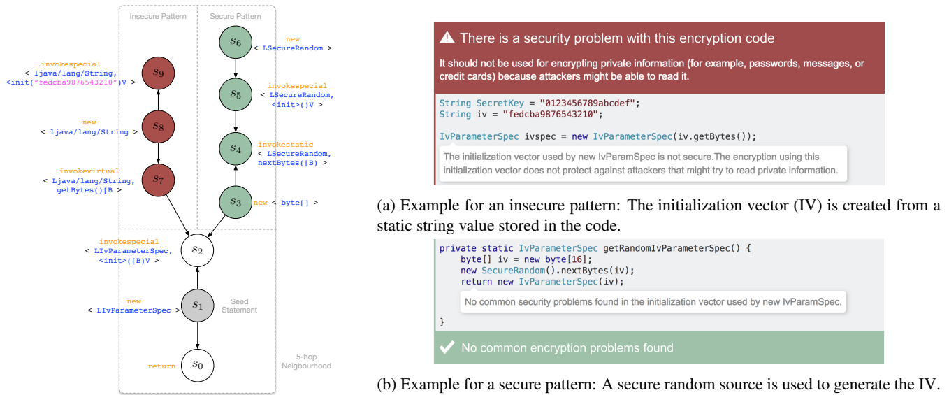
Figure 2: Example for a secure and insecure usage pattern of new IvParameterSpec . It shows the program dependency graph (PDG) of the 5-hop neighborhood of the seed statement s_1 for the secure and insecure code example displayed in (a) and (b). Next to each node in the graph we provide the shortened signature of the related statement, highlighting a subset of its attributes we store in the feature vector. Bytecode instruction types are highlighted yellow, Java types and constants magenta.
