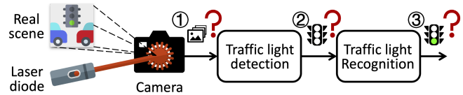
Figure 2: Illustration of the three attack stages.
