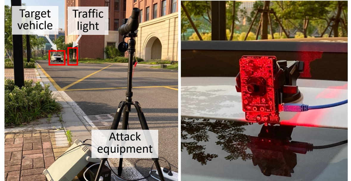
Setup for long-range laser aiming experiment (the attacker was on the roadside and 40-80 m away from the vehicle)
