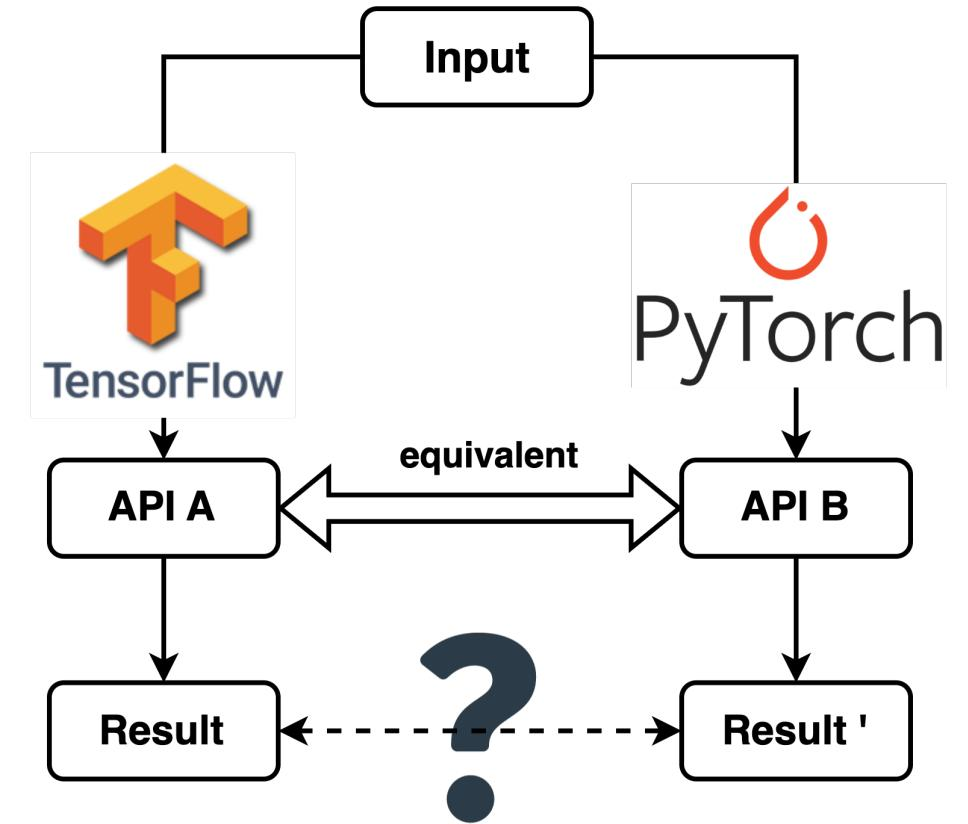
Using differential testing for cross deep learning framework testing.
