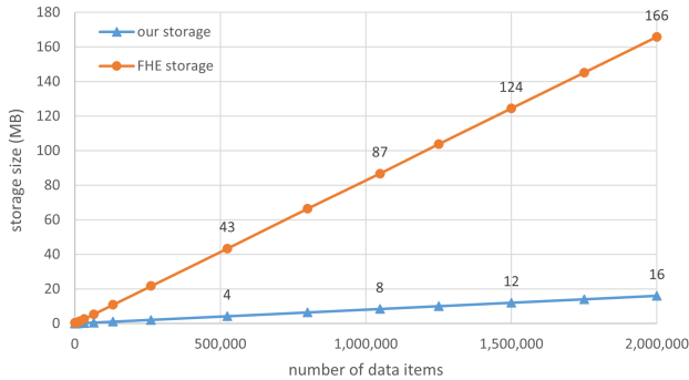
(a) Storage size (MB) in our solution vs. baseline, on data items encrypted one-by-one (top) or in batched form (bottom)
