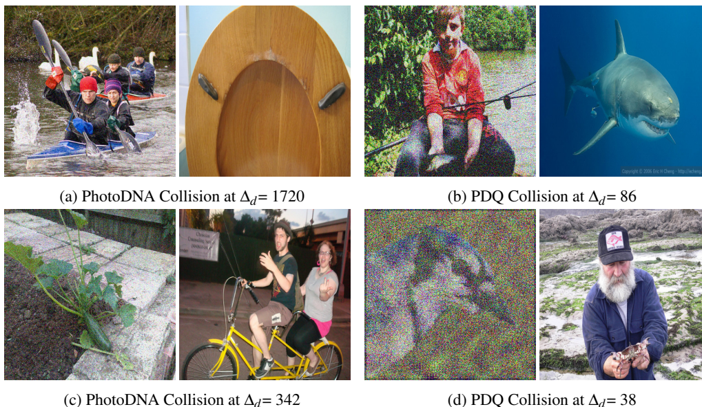
Figure 1: Targeted-second-preimage collision pairs for PhotoDNA and PDQ at high (top) and low (bottom) matching thresholds. The image on the left in a pair is our attack image, while the image on the right is the target. A lower matching threshold implies a better collision, potentially at the cost of image quality. Each pair was generated as described in Section 4.1.
