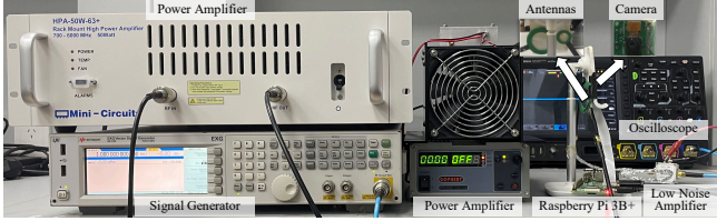
Figure 16: Illustrations of the experimental setup for investigating the performance of GlitchHiker attack.
