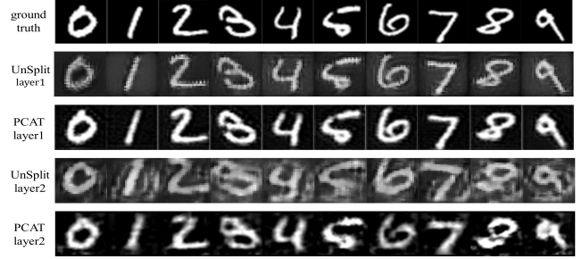
Figure 17: Input data reconstruction results of PCAT and UnSplit [9] on MNIST. In PCAT, the server attacks using 5 samples per class from X_{priv} for layer1 and 10 samples per class for layer2.
