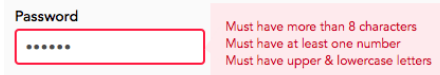
(c) A 3class8 character-class PCP, which requires passwords be at least 8 characters in length with at least 1 lowercase, 1 uppercase, and 1 number.
