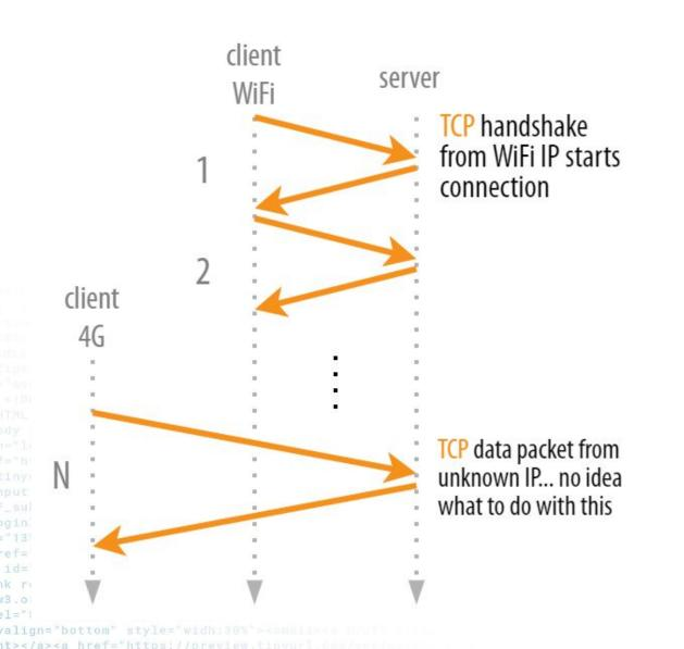
All client TCP connections need to be re-established after 4-tuple changes
