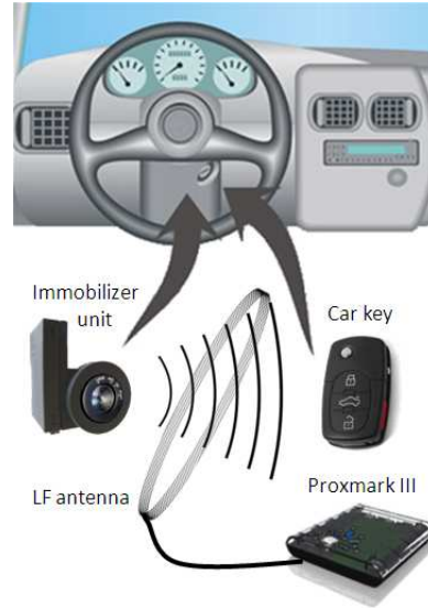
Figure 5: Experimental setup for eavesdropping
