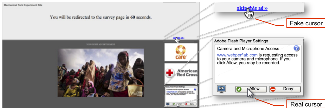
Figure 1: Cursor spoofing attack page. The target Flash Player webcam settings dialog is at the bottom right of the page, with a “skip this ad” bait link remotely above it. Note there are two cursors displayed on the page: a fake cursor is drawn over the “skip this ad” link while the actual pointer hovers over the webcam access “Allow” button.
