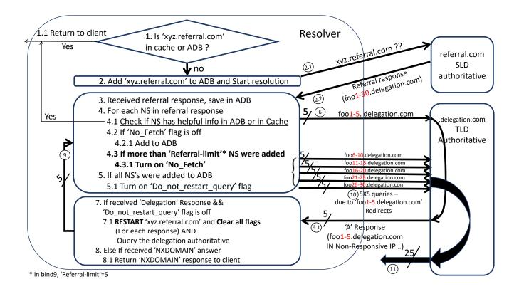
Figure 2: Delegation server variant of the NRDelegationAttack flowchart; the resolver resolution algorithm during the attack.
