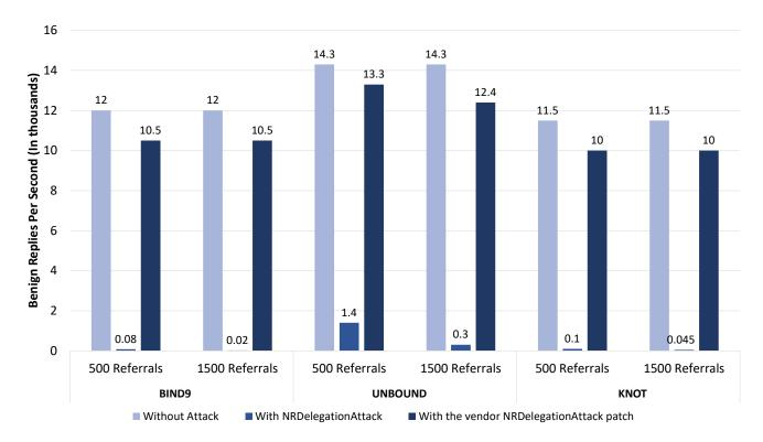
Figure 7: Resolver throughput during NRDelegationAttack, tested on NRDelegationAttack patched and non-patched versions of BIND9, Knot, and Unbound implementations.
