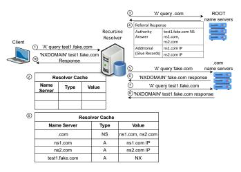
Figure 10: Querying the authoritative chain using QNAME Minimisation and saving the result in the resolver cache.
