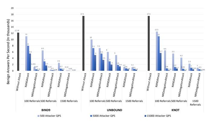
Figure 5: Resolver throughput tested on NXNSAttack patched versions of BIND9, Knot, and Unbound implementations under and without either NRDelegationAttack or NXNSAttack.
