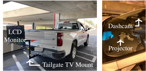
Figure 7: Real-world experiment setup. (Left) An LCD monitor is mounted on the back of the front vehicle. (Right) A dash-cam is mounted on the windshield of the ego vehicle. A portable projector is taped on the dashboard.
