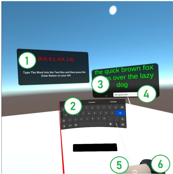
Figure 7: Data collection app. (1) The background app records the sensor readings even it is not in focus. The user types into the foreground keyboard (2), following the sentence prompt (3), in the text field (4). (5) The system hand controller is used to type, but the background app only has access to the (6) application hand controller, which is frozen while the keyboard is in focus.
