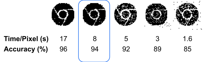
Figure 20: Results for pixel stealing on AMD RX 6600, with varying amounts of sampling period per pixel. The baseline period of 8 seconds is highlighted.
