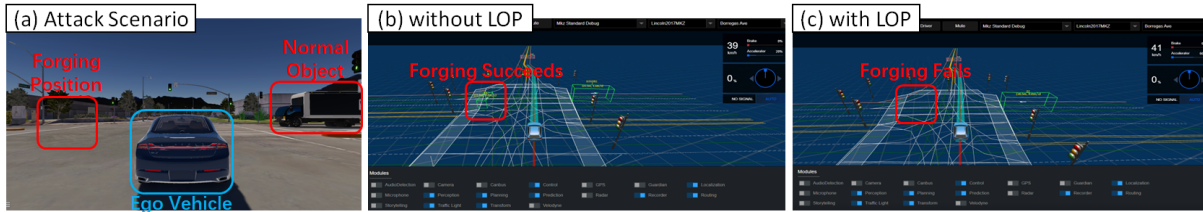
Figure 7: The simulating scenario and the Dreamview of Apollo 6.0.0 without and with our LOP under Physical attack.
